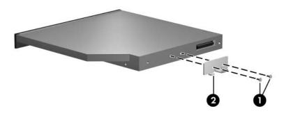
Removing the Optical Drive Bracket
