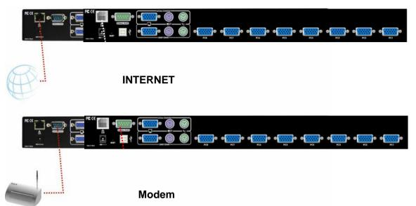
The rear side of DKVM-IP8 switch provides a RJ-45 connector for Ethernet. The connector is used either for a 100 Mbps 100BASE-TX connection or for a 10 Mbps 10BASE -T connection. The adapter can sense the connection speed and will adjust to the appropriate operation mode automatically.
